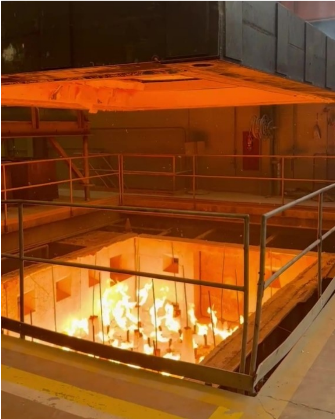
DSI-HHS10B Horizontal Fire Curtain- Furnance Test
