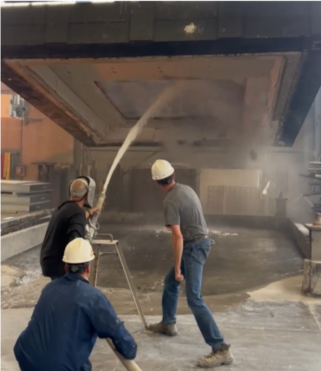
DSI-HHS10B Horizontal Fire Curtain- Enduring Hose Stream Test
