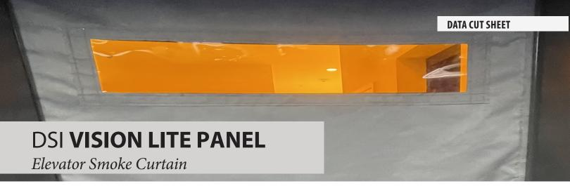
The Elevator Smoke Containment System by Door Systems Model DSI-600 is designed to offer reliable performance in case of a fire. The curtain is hidden inside a compact head-box when not in use, but it is triggered by the Fire Alarm and quickly deploys to contain smoke. The DSI-600 system complies with IBC and NFPA standards and can be used as an alternative to elevator lobbies. Working in tandem with the fire-rated hoistway doors to ensure maximum safety.
